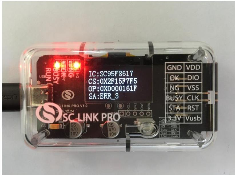
Figure 1.2.4-2 Programming Failed with Limited Counts Used Up
