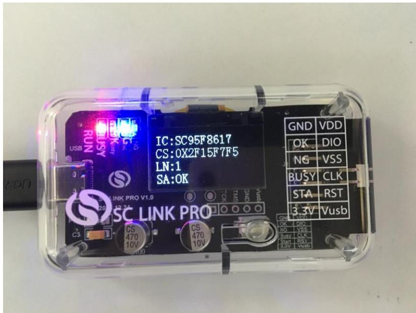
Figure 2.2.4-1 Programming with Limited Counts Completed
