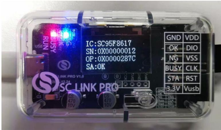
Figure 2.2.3-2 SC LINK PRO S/N Offline Programming Completed
