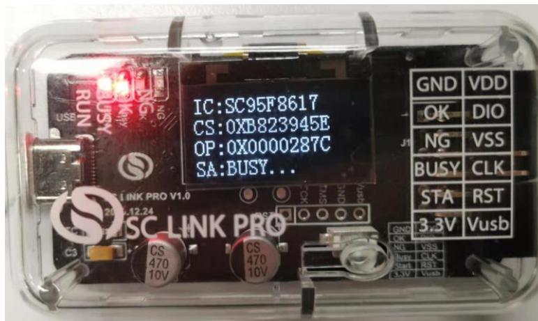
Figure 2.2.3-1 SC LINK PRO S/N Offline Programming in Progress
