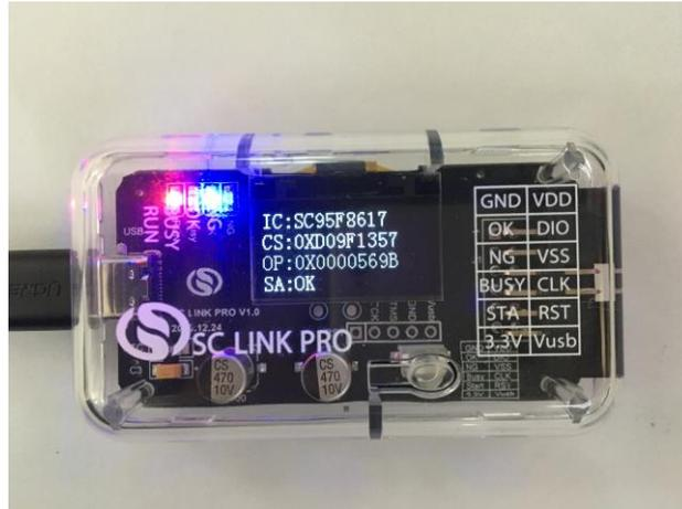
Figure 2.2.2 SC LINK PRO Display under Conventional Offline Programming
